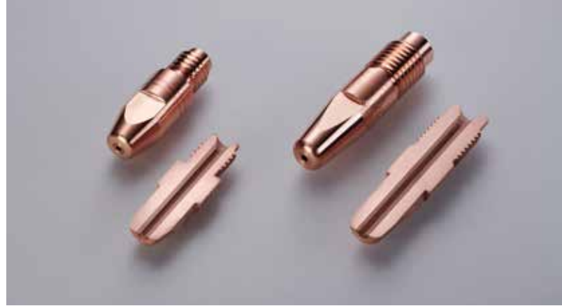
Contact tips made of CEP DISCUP®+Cu composite tube. The longitudinal cross-section shows the CEP DISCUP® core surrounded by a copper sheath
